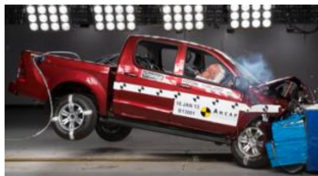
Frontal offset test at 64 km/h
